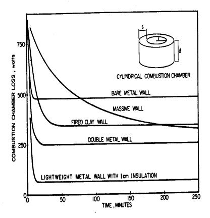
double wall construction can dramatically lower heat loss (Figure 4B). Materials such as sand-clay or concrete, which have a high specific heat and density, and which must be formed in thick sections to be sufficiently strong to support a pot or resist the fire, should therefore be avoided. Heat Recuperation It has frequently been argued that the large amounts of heat absorbed by the walls of a massive stove should be utilized by either extinguishing
