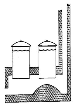
Figure 1c: Two pot massive wood stove with chimney.
