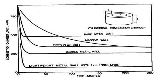
FIGURE 4B: Heat loss into and through combustion chamber walls of varying materials as a function of time elapsed since starting the fire
