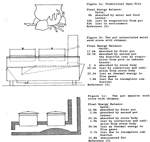
stoves much of the heating potential of this gas is lost (Figure 1). Increasing convective heat transfer to the pot is the single most important way to increase the thermal efficiency of a woodburning stove.
