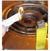
**Using a match**: strike the match and drop it down into the combustion chamber.
