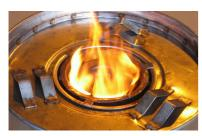
When the paraffin enters the hot heater pipe, it will make a rushing sound as the gas leaves the jet and burns under the bluff plate. During this time the heater pipe continues to increase in temperature and the flame is not stable. If you open the fuel control valve at just the right time, the fire will not smoke at all.
