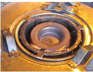
As the spirits flame dies out the paraffin takes over. Until the spirits is burned completely, the paraffin flame will be disturbed. Here is a picture of the paraffin flame just after the spirits burned away. Notice it is partly blue and mostly yellow. The heater pipe will still get hotter for a few more minutes.
