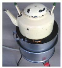
Put the heat shield into place atop the stove. The heat shield can get quite hot so always use the handle. The heat shield increases the upward draft on the flames and in some cases, removing the pot while the heat is on HIGH can actually suck the flame up and it auto-extinguishes. Before lifting out the pot, turn the fuel control valve to mid-range.
