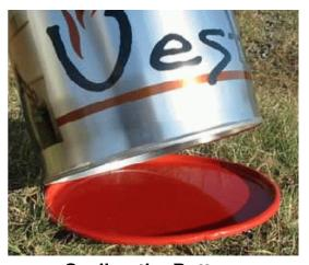
Sealing the Bottom If the stove is placed on a flat surface like a cement floor then the bottom is sealed and air does not get under the side. This is correct Air should not be able to get to the fire except through the holes in the side. If the ground is very soft you can press the Vesto downwards gently while rotating it which will cause the bottom to sink in and create a seal.
