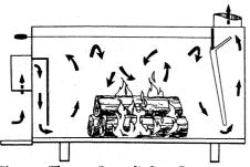
Fig. 67. Thermo-Control's heat-flow pattern.
