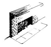
Fig. 4. From 40 to 60 percent of latent heat goes up the fireplace chimney as dark, smoky gases. deal with this problem in a variety of ways (to be discussed in chapter 2) and with varying degrees of success (Fig. 5).
