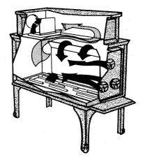
Fig. 8. Cutaway view of Nordic stove with flip-open damper and contoured side baffles.
