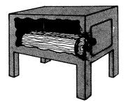
Fig. 10. Cut logs 2 inches shorter than the depth of your stove's firebox.
