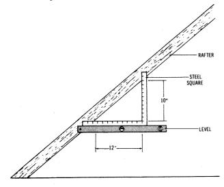
Fig. 8. Measuring roof pitch, using level and steel square.
