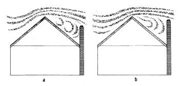
Fig. 6. Chimney height too low (a) causing back-puffing. Correct height shown at (b).
