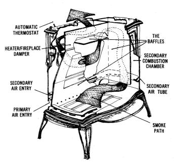
Fig. 12. Cutaway view of the Defiant stove.
