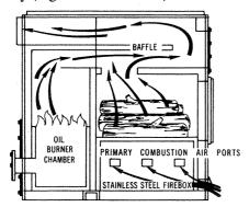
Fig. 79. Hunter combination wood/oil furnace flow-patterns.
