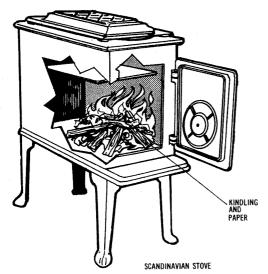
Fig. 3. Kindling burned in front part of firebox and logs added later.
