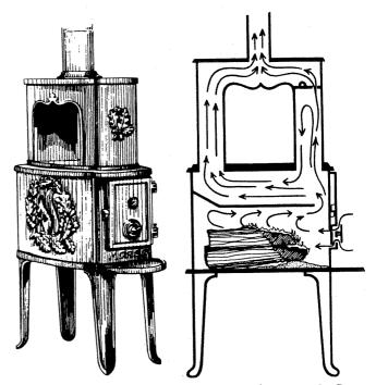
Fig. 16. Morsø Model 1BO box stove (left) showing smoke flowpattern and baffle system (right).
