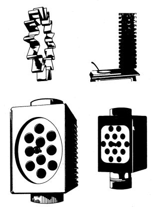
Fig. 6. Items used to increase heat radiation from stovepipe.
