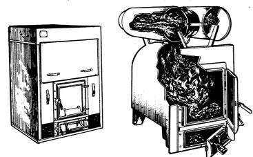
Fig. 77. Daniels wood-burning furnace (left) showing interior view (right).
