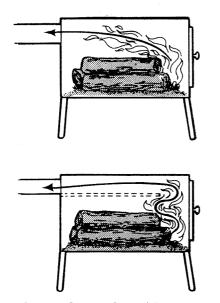
Fig. 2. Direct flame-path in traditional box stove versus "S"shaped flame-path in Scandinavian baffled stove.
