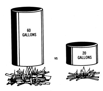
Fig. 2. Takes more heat to raise 60 gallons one degree than 20 gallons one degree.
