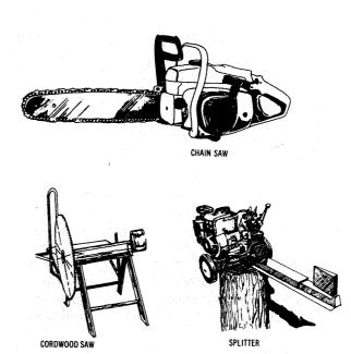
Fig. 3. Power tools for cutting and splitting firewood.
