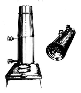
Fig. 1. Stovepipe water heater.
