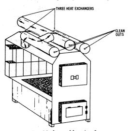
Fig. 82. Ray-Mask wood-burning furnace.
