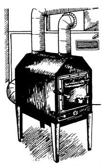
Fig. 84. Lumberjack add-on wood-burning furnace.
