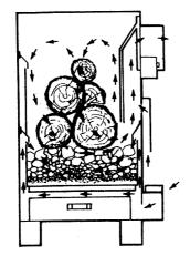
Fig. 11. Air-flow pattern in the Riteway 2000.
