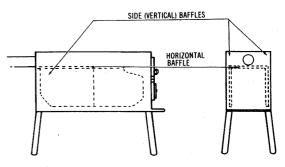
Fig. 1. Scandinavian woodstove interior baffle arrangement from side (left) and front (right).
