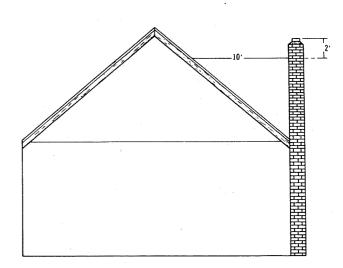
Fig. 5. Chimney height in relation to 10-foot distance from roof.
