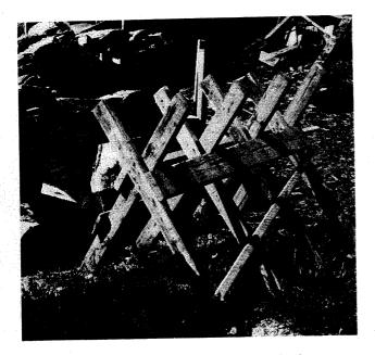
Fig. 5. Home-made, heavy-duty sawbuck.
