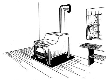
Fig. 60. Hydrostove step stove for hot-water system.
