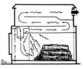
Fig. 6. Flow-pattern and baffle arrangement in Home Warmer stove.
