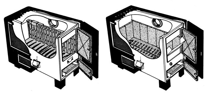
Fig. 23. Cutaway views of Homesteader circulating heaters, Model 240 (left) and Model 240DG (right).
