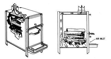
Fig. 63. Greenwood (left) and Double Dynamite (right).
