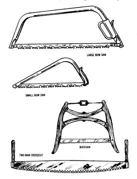
Fig. 4. Tools for cutting wood by hand.
