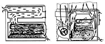
Fig. 80. Valley Comfort wood-burning furnace flow-patterns.
