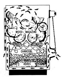
Fig. 25. Valley Comfort automatic circulating heater, showing flow-patterns.
