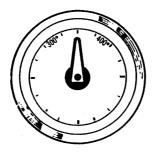
Fig. 6. Stack temperature should be 300-400 degrees F.
