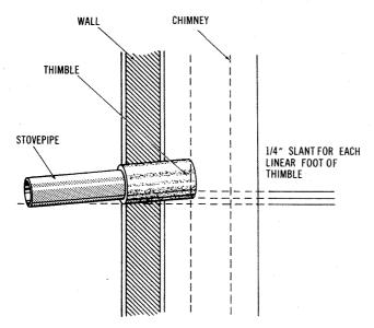
Fig. 17. Angle of thimble from horizontal.
